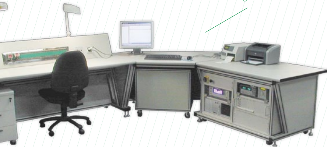
Electrical and functional testing table for high tension
